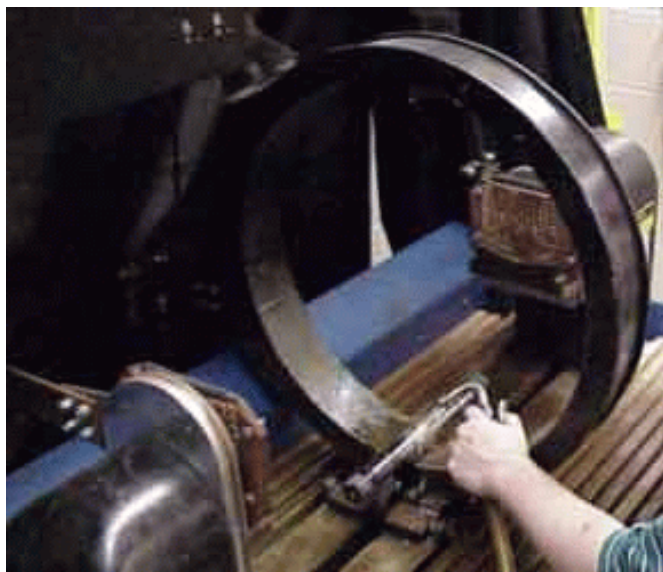
figuur 4.8 Indirecte methode van as in spoel ( http://www.ndt-ed.org )
